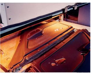
Infrared heat activates adhesives on decorative trims Medium wave infrared emitters perfectly activate the adhesive for plastic decorative trims on door panels.
